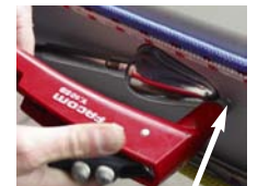
fixing a safety rivet
