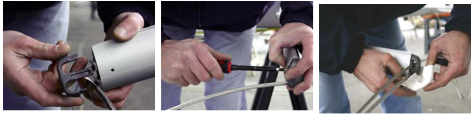
Check the positioning of the cables before fixing the tips of the spreaders
