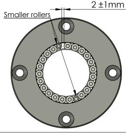
6. The extra space between rollers should be 2mm ±1mm, and when the extra space is not within the tolerance, you should take out 1 or 2 rollers and add smaller rollers.
