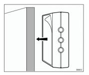
3. Alternatively, the PC/SeaTalk/NMEA Interface box may be attached using the 2 self tapping screws provided.
