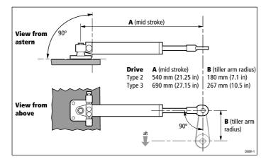
Figure 4: Hydraulic ram alignment
