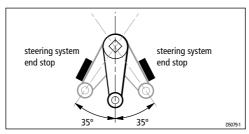
Figure 8: Total rudder movement
