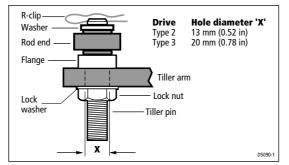
Figure 7: Attaching the push rod to the tiller arm
