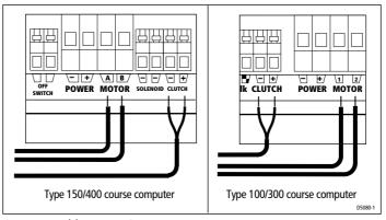
Figure 9: Cable connections at course computer
