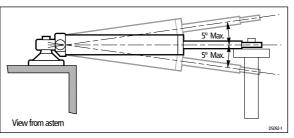
Figure 5: Alignment between push rod and tiller arm plane of rotation
