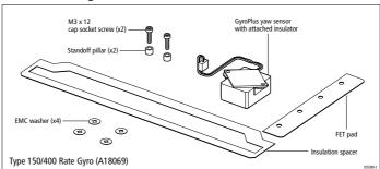
Figure 1: Contents of Rate Gyro assembly kit
