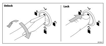
Figure 3: Unlocking and locking the connector cover
