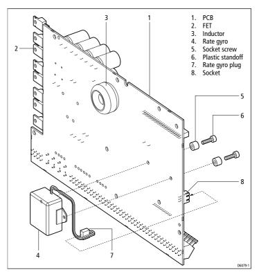
Figure 7: Installation of the GyroPlus yaw sensor
