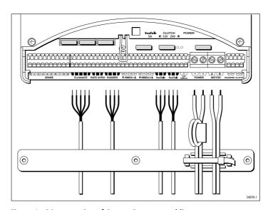
Figure 4: Disconnection of Course Computer cabling
