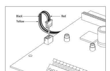
Figure 8: Rate Gyro Connector Orientation
