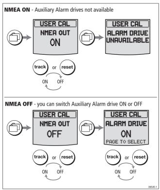
5. When you have set NMEA OUT and ALARM DRIVE as required, hold down the 🗇 and 🗊 buttons for approximately 2 seconds to return to normal operation.
